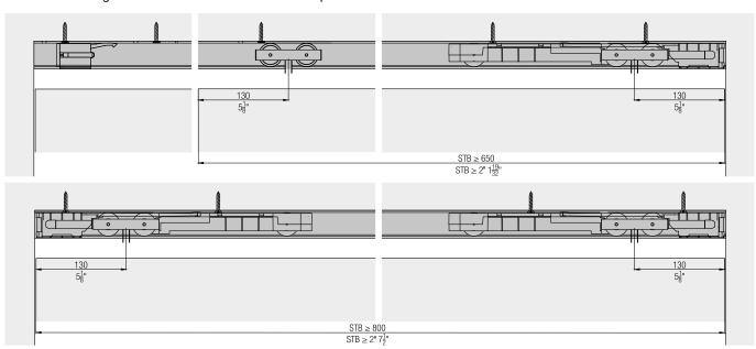
Fitting for top-running glass doors up to 100 kg (220 lbs.), with surface mounted running track or running track flush with the ceiling. Optionally with soft and self closing mechanism. Ceiling mounting. Minimal installation height. Wall pocket solution.
