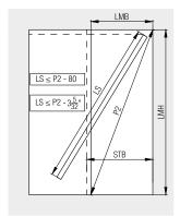
LMB = inside clearance LMH = inside height STB = sliding door width P2 = diagonal clearance LS = running track
